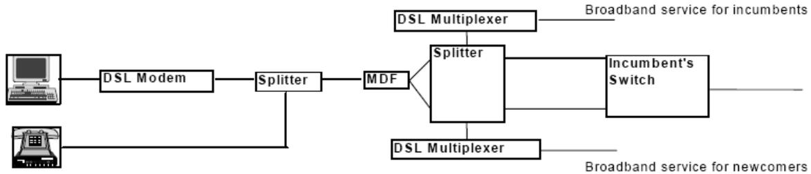
Thus, Bit Stream Access is a wholesale product consisting of the access (typically ADSL) and “backhaul” services of the (data) backbone network (ATM, IP backbone).
