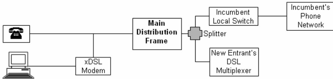
Line sharing allows the incumbent to continue to provide telephone service while the competitor provides broadband (xDSL) services on the same copper pair. With line sharing, the competing supplier uses the non-voice frequency of the loop. Consumers can obtain broadband service from the most competitive provider without installing a second line.
